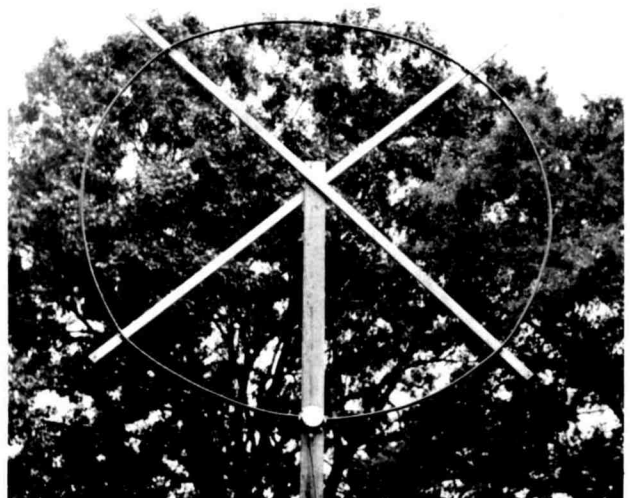
The coaxial loop of fig. 4 as built by the author.
